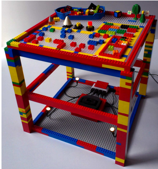
Figure 2. Case study: a tangible rhythm sequencer with parameter controls. The translucent top surface of the table is covered with different types of widgets. A high definition camera and illumination are mounted underneath.
